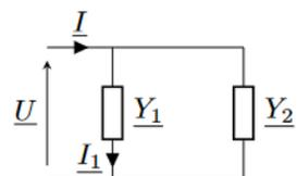
$$\begin{cases} \underline{I} = (\underline{Y}_1 + \underline{Y}_2) \underline{U} \\ \underline{I}_1 = \underline{Y}_1 \underline{U} \end{cases} \quad \text{donc} \quad \boxed{\frac{\underline{I}_1}{\underline{I}} = \frac{\underline{Y}_1}{\underline{Y}_1 + \underline{Y}_2}}$$
