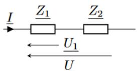
$$\begin{cases} \underline{U} = (\underline{Z}_1 + \underline{Z}_2) \underline{I} \\ \underline{U}_1 = \underline{Z}_1 \underline{I} \end{cases} \quad \text{donc} \quad \boxed{\frac{\underline{U}_1}{\underline{U}} = \frac{\underline{Z}_1}{\underline{Z}_1 + \underline{Z}_2}}$$
