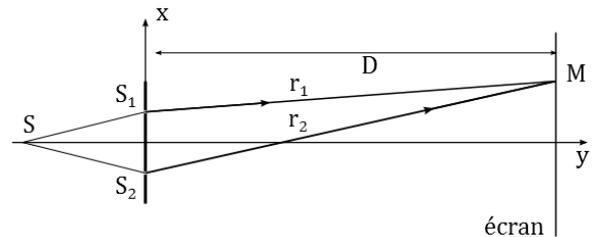
$$I(M) = \frac{1}{2} \underline{s} \cdot \underline{s}^* \quad I_1 = \frac{1}{2} s_1^2 \quad I_2 = \frac{1}{2} s_2^2 \quad \text{d'où } I_1 I_2 = \frac{1}{4} s_1^2 s_2^2 \quad \text{soit } s_1 s_2 = 2\sqrt{I_1 I_2}$$
