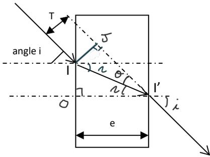
1) Considérations géométriques :  $\left. \begin{array}{l} \text{triangle } I J I' \\ \sin(\theta) = \frac{T}{II'} \end{array} \right\} \text{ et } \left. \begin{array}{l} \text{Triangle } O I I' \\ \cos(r) = \frac{e}{II'} \end{array} \right\}$
