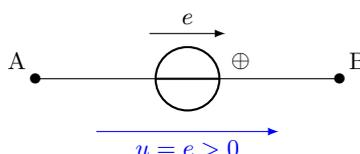
FIGURE 16 – Source idéale de tension.
