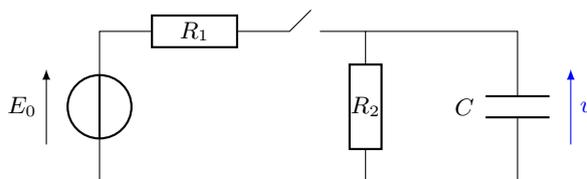
$$R_1 = 330 \text{ k}\Omega \quad C = 0,10 \text{ }\mu\text{F}$$
