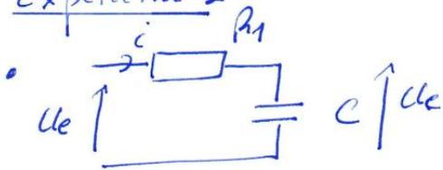
$$\left. \begin{aligned} U_e &= R_1 i + U_c \\ i &= C \frac{dU_c}{dt} \end{aligned} \right\} U_e = R_1 C \frac{dU_c}{dt} + U_c$$
