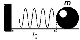
$$\begin{aligned} \vec{P} + \vec{F} + \vec{R} + \vec{f} &= m\vec{a} \\ -kx - \alpha\dot{x} &= m\ddot{x} \\ \ddot{x} + \frac{\omega_0}{Q}\dot{x} + \omega_0^2x &= 0 \end{aligned}$$
