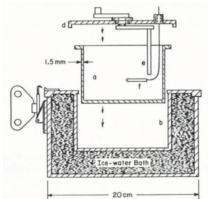
Fig. 1. Polycarbonate calorimeter for measurement of the liquid water content of snow: (a) reaction cup, (b) air space, (c) ice-water bath, (d) reaction-cup cover, (e) stirrer, (f) resistance temperature detector.
