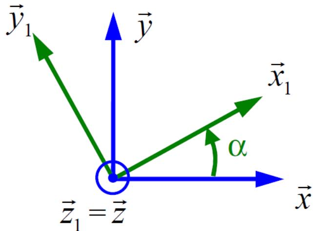
$$\vec{V}(A \in 1/0) = \left( \frac{d\overrightarrow{OA}}{dt} \right)_0 = \left( \frac{d(R \cdot \vec{y}_1)}{dt} \right)_0 = R \left( \frac{d\vec{y}_1}{dt} \right)_0$$
