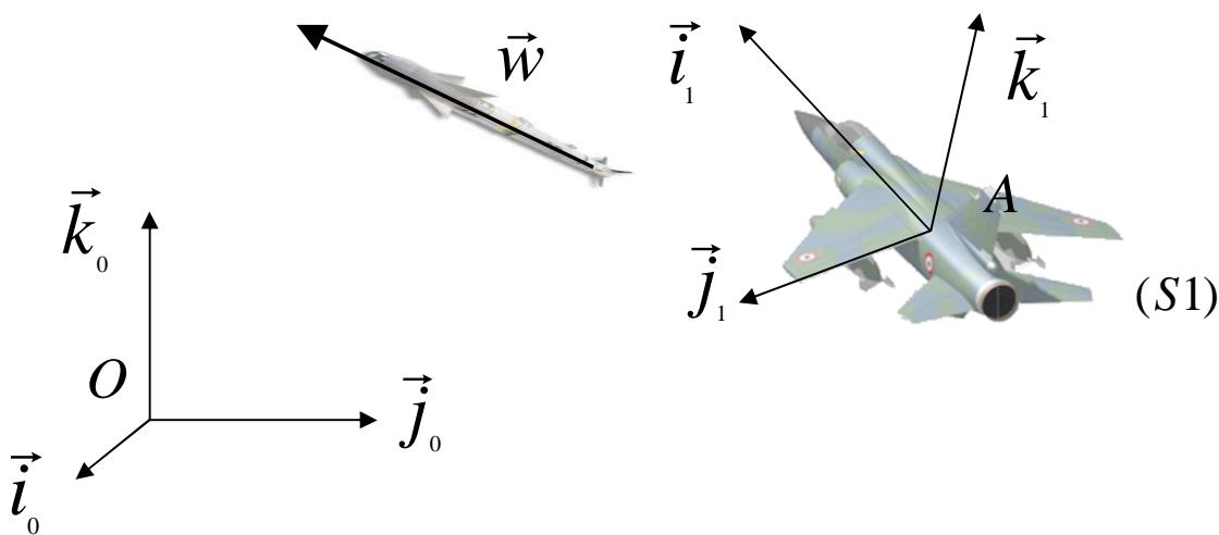
$$\text{Formule de la base mobile : } \left( \frac{d\vec{w}}{dt} \right)_{R_0} = \left( \frac{d\vec{w}}{dt} \right)_{R_1} + \vec{\Omega}(R_1 / R_0) \wedge \vec{w}$$
