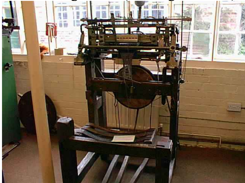
A stocking-frame (knitting machine)
