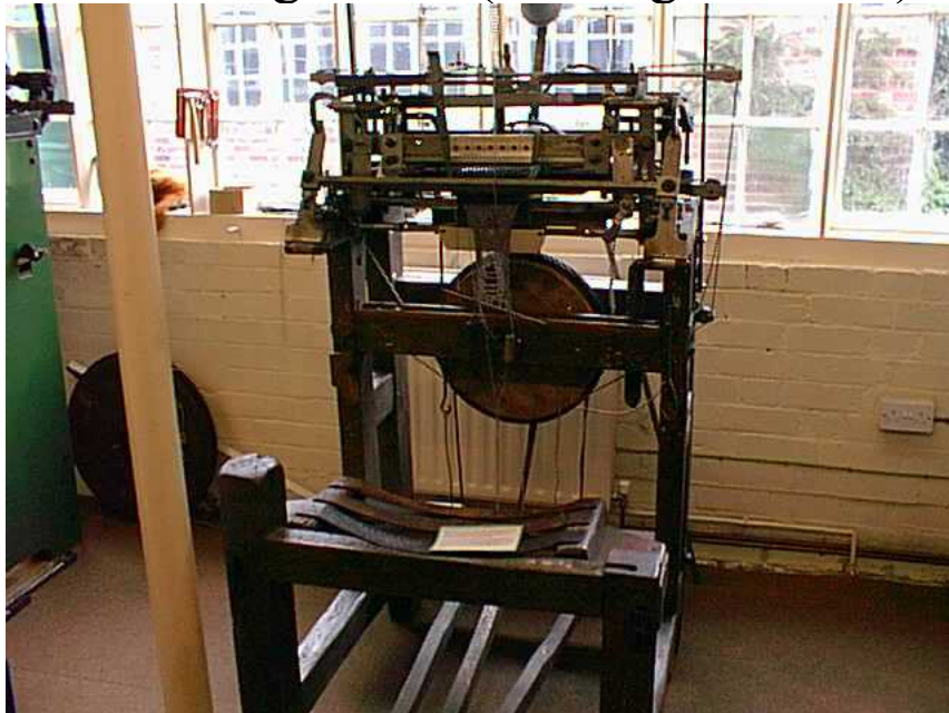
A stocking-frame (knitting machine)
