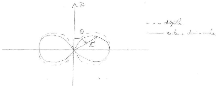
$$\textcircled{2} \quad P = \iint_{\text{sph}} \langle \vec{R} \rangle \cdot \vec{n} \, dS = \frac{\mu_0 I_0^2 c}{8\pi^2} \int_{\theta=0}^{\pi} \int_{\varphi=0}^{2\pi} \frac{\cos^2\left(\frac{\pi}{2} \cos\theta\right)}{r^2} r^2 \sin\theta \, d\theta \, d\varphi$$
