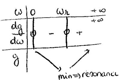
$$\omega_r = \omega_0 \sqrt{1 - \frac{1}{2Q^2}} \quad \left. \begin{array}{l} \text{pour} \\ Q > \frac{1}{\sqrt{2}} \end{array} \right\}$$
