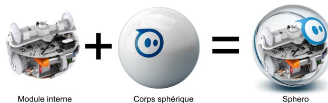
Figure 1 Constitution du Sphero
