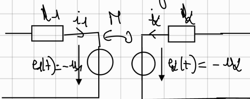
$$e_1(t) = -\frac{d\Phi_1}{dt} \quad \text{avec } \Phi_1 = L_1 i_1 + M i_2$$
