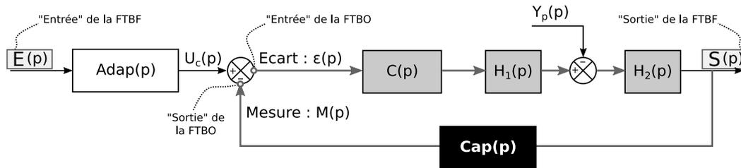
$$FTBF(p) = \left. \frac{S(p)}{E(p)} \right|_{Y_p(p)=0} = \dots\dots\dots$$
