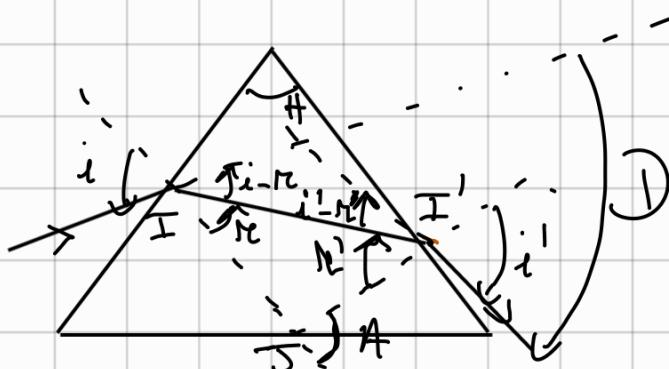
$$\begin{aligned} a - \underline{\sin i = n \sin r} \\ \underline{\sin i' = n \sin r'} \end{aligned}$$
