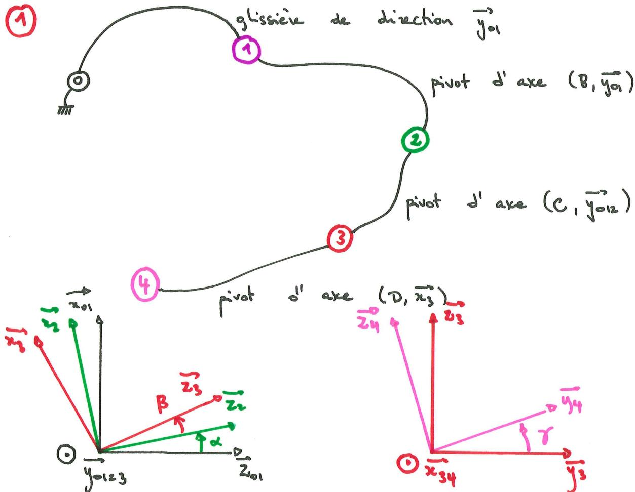
$$\textcircled{2} \quad \vec{J}_{PE4/0} = \vec{J}_{PE4/3} + \vec{J}_{PE3/2} + \vec{J}_{PE2/1} + \vec{J}_{PE1/0}$$
