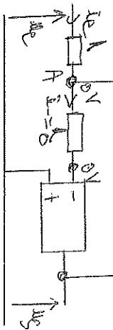
$$\begin{aligned} U_{\text{in}} &= U_A = 0 \\ I_{\text{in}} &= 0 \quad U_{\text{out}} = U_A = 0 \\ \text{On a alors } &\text{ le feedback} \\ \text{neutre sur } &\text{H:} \\ U_{\text{in}} &= - \frac{U_{\text{out}}}{A_H} \Rightarrow U_{\text{out}} = - U_{\text{in}} \end{aligned}$$
