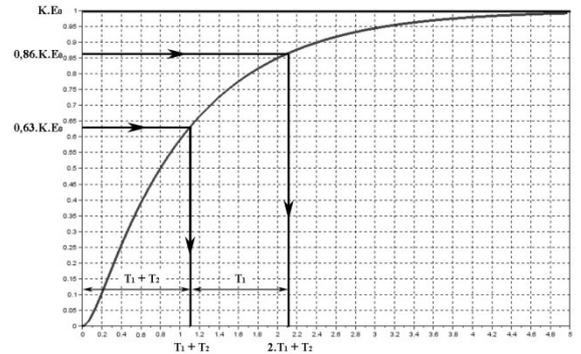
$$s'(t) = \frac{K.E_0}{T_1 - T_2} \cdot \left( e^{-t/T_1} - e^{-t/T_2} \right)$$
