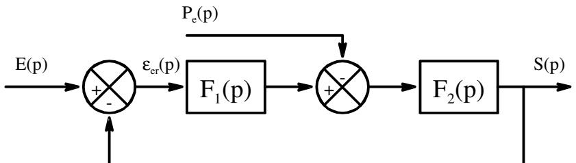
$$F_1(p) = \frac{K_1}{p^{\alpha_1}} \cdot \frac{N_1(p)}{D_1(p)} \quad \text{et :} \quad F_2(p) = \frac{K_2}{p^{\alpha_2}} \cdot \frac{N_2(p)}{D_2(p)}$$
