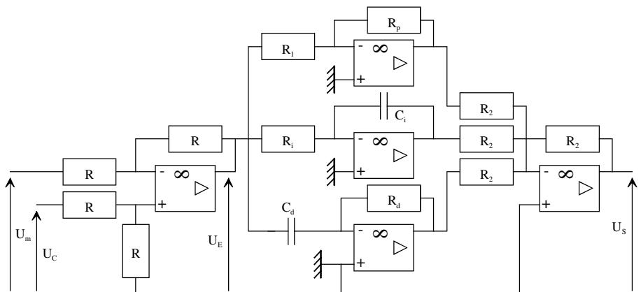
$$U_s(t) = \frac{R_p}{R_1} \cdot U_E(t) + \frac{1}{R_i \cdot C_i} \int U_E(t) \cdot dt + R_d \cdot C_d \cdot \frac{d U_E(t)}{dt}$$
