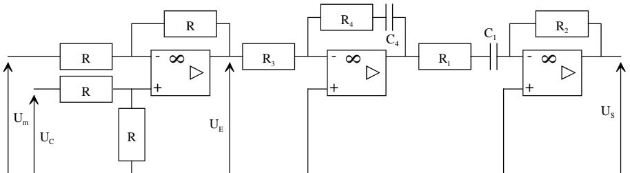
$$C(p) = \frac{1 + R_4.C_4.p}{R_3.C_4.p} \cdot \frac{R_2.C_1.p}{1 + R_1.C_1.p} = \frac{\frac{R_2.C_1}{R_3.C_4} \cdot \left( 1 + \frac{R_4.C_4}{R_1.C_1} \cdot R_1.C_1 \cdot p \right)}{1 + R_1.C_1 \cdot p}$$
