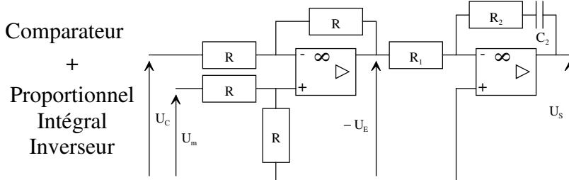
$$u_s(t) = \frac{R_2}{R_1} \left( u_E(t) + \frac{1}{R_2 \cdot C_2} \int u_E(t) \cdot dt \right)$$
