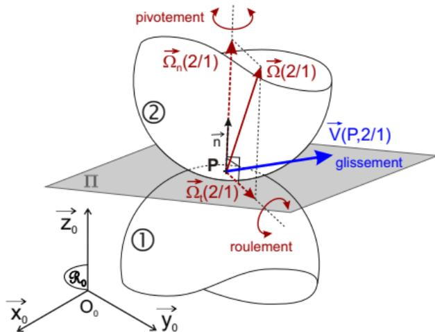
$$\left\{ \mathcal{V}_{(2/1)} \right\} = \left\{ \begin{array}{l} \vec{\Omega}_{(2/1)} = \vec{\Omega}_n(2/1) + \vec{\Omega}_t(2/1) \\ \vec{V}(P, 2/1) \end{array} \right\}_P$$
