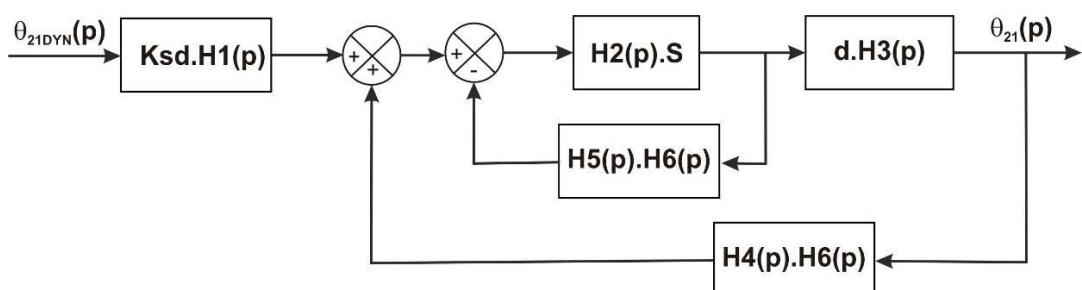
$$F_{DYN}(p) = \frac{\theta_{21}(p)}{U(p)} = \frac{\theta_{21}(p)}{\theta_{21DYN}(p)} = K_{sd}H_1(p) \frac{d \cdot H_3(p) \frac{H_2(p) \cdot S}{1 + H_2(p) \cdot S \cdot H_5(p) \cdot H_6(p)}}{1 - d \cdot H_3(p) \frac{H_2(p) \cdot S}{1 + H_2(p) \cdot S \cdot H_5(p) \cdot H_6(p)} H_4(p) \cdot H_6(p)}$$
