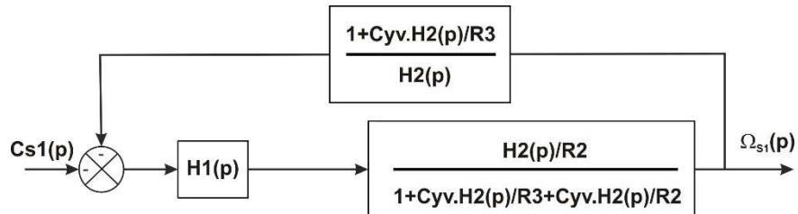
$$F_1(p) = \frac{\Omega_{S1}(p)}{C_{S1}(p)} = -\frac{H_1 H_2 / R_2}{1 + C_{yV} H_2 / R_3 + C_{yV} H_2 / R_2 + H_1 / R_2 (1 + C_{yV} H_2 / R_3)}$$
