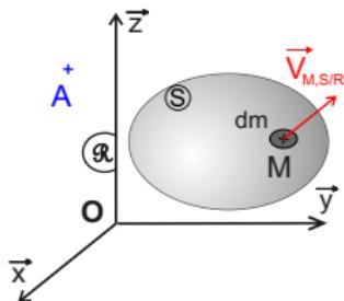
$$\vec{\delta A}(S/R) = \left. \frac{d\vec{\sigma}_{A(S/R)}}{dt} \right|_R + \int_{M \in S} \vec{V}_{(A/R)} \wedge \vec{V}_{(M,S/R)} dm$$
