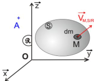
$$\left\{ \mathcal{C}_{(S/R)} \right\} = \left\{ \begin{array}{l} \vec{R}_{c(S/R)} = \int_{M \in S} \vec{V}_{(M,S/R)} \cdot dm = \mathbf{m}_S \cdot \vec{V}_{(G,S/R)} \\ \vec{\sigma}_{A(S/R)} = \int_{M \in S} \vec{AM} \wedge \vec{V}_{(M,S/R)} \cdot dm \end{array} \right\}_A$$
