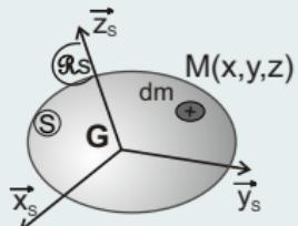
$$\mathbf{I}(G, S) = \begin{bmatrix} \int_{M \in S} (y^2 + z^2).dm & \int_{M \in S} -xy.dm & \int_{M \in S} -xz.dm \\ \int_{M \in S} -xy.dm & \int_{M \in S} (x^2 + z^2).dm & \int_{M \in S} -yz.dm \\ \int_{M \in S} -xz.dm & \int_{M \in S} -yz.dm & \int_{M \in S} (x^2 + y^2).dm \end{bmatrix}_{\mathcal{B}_s}$$
