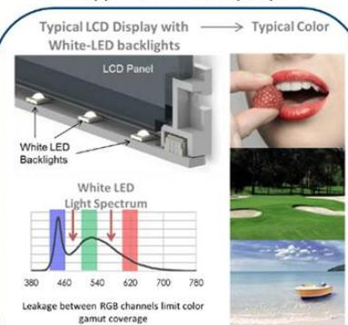
Leakage between RGB channels limit color gamut coverage
