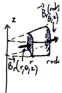
$$\begin{aligned} \Phi_{2(\text{selon } \vec{u}_\theta)} &= B_\theta(r, \theta, z) dr dz - B_\theta(r, \theta+d\theta, z) dr dz \\ &= -\frac{\partial B_\theta}{\partial \theta} d\theta dr dz \\ &= -\frac{1}{r} \frac{\partial B_\theta}{\partial \theta} d\mathcal{V} \end{aligned}$$
