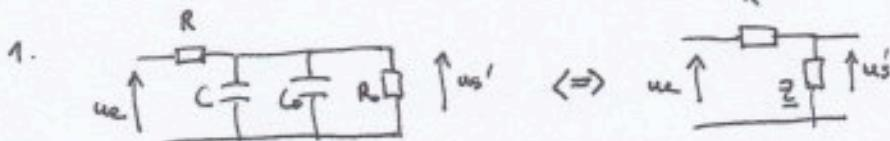
$$\text{avec } \underline{\frac{Z}{R}} = \frac{R_o \times \frac{1}{f\omega(C+L_o)}}{R_o + \frac{1}{f\omega(C+L_o)}} = \frac{R_o}{1 + f\omega R_o(C+L_o)}$$
