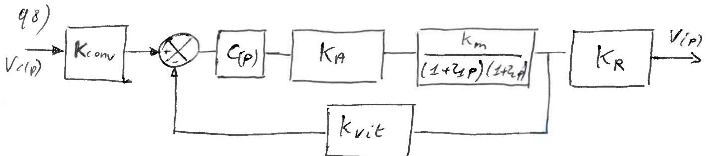
$$99) H(p) = \frac{V(p)}{V_c(p)} = K_{\text{conv}} K_R \cdot \frac{\frac{C(p) K_A \frac{K_m}{(1+z_1 p)(1+z_2 p)}}{1 + \frac{C(p) K_A K_m K_{\text{rit}}}{(1+z_1 p)(1+z_2 p)}}}$$
