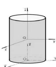
$$\overline{I}_G = \begin{bmatrix} \frac{m}{12}(3R^2+h^2) & 0 & 0 \\ 0 & \frac{m}{12}(3R^2+h^2) & 0 \\ 0 & 0 & \frac{m}{2}R^2 \end{bmatrix}_{(x,y,z)}$$
