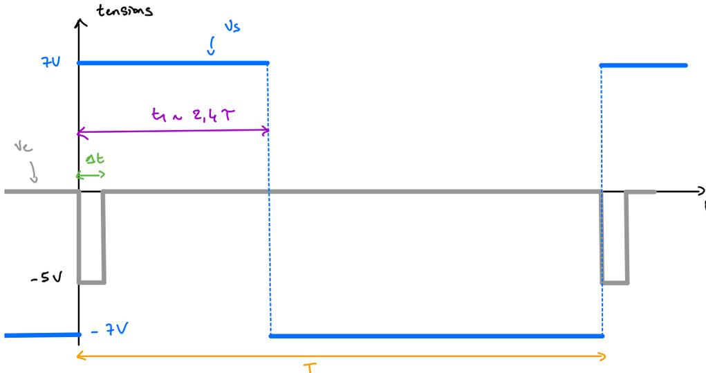
19.  $\langle V_s \rangle = V_{sat} \frac{2t_1 - T}{T} = V_{sat}(2ft_1 - 1)$
