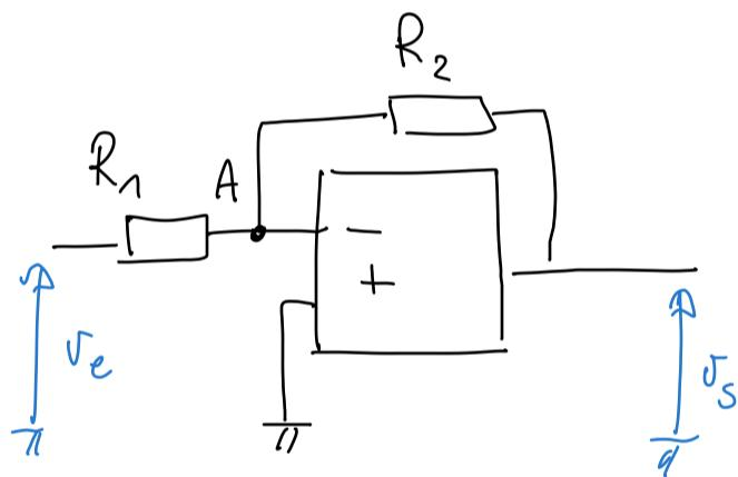
$$\left. \begin{array}{l} V^+ = 0 \\ V^- = V_A \end{array} \right\} \Rightarrow V_A = 0$$
