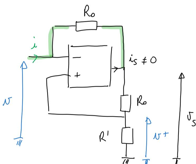
$$\begin{cases} u^- = u \\ u^+ = \frac{R'}{R' + R_o} u_s \end{cases} \quad \left. \begin{array}{l} \\ \end{array} \right\} u_s = \left( 1 + \frac{R_o}{R'} \right) u$$
