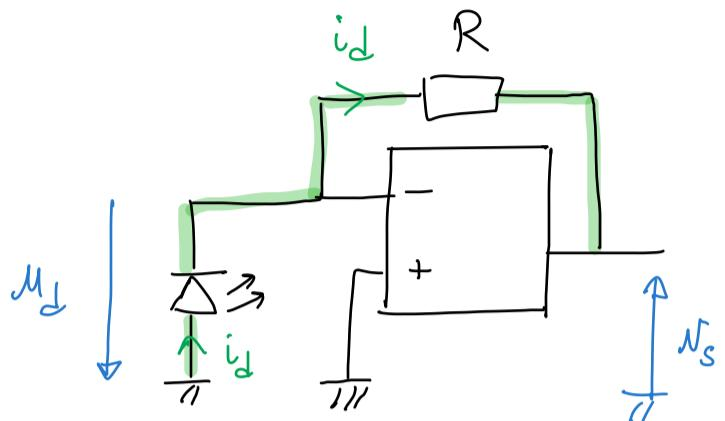
$$\begin{aligned} u^+ &= 0 \\ u^- &= u_d \end{aligned} \quad \left. \begin{array}{l} \\ \end{array} \right\} M_d = 0$$
