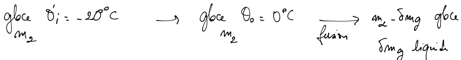
$$\Delta S_{gba} = m_2 c_g \ln \left( \frac{T_o}{T_i} \right) + \delta_{mg} \frac{\ell_{fus}}{T_o}$$
