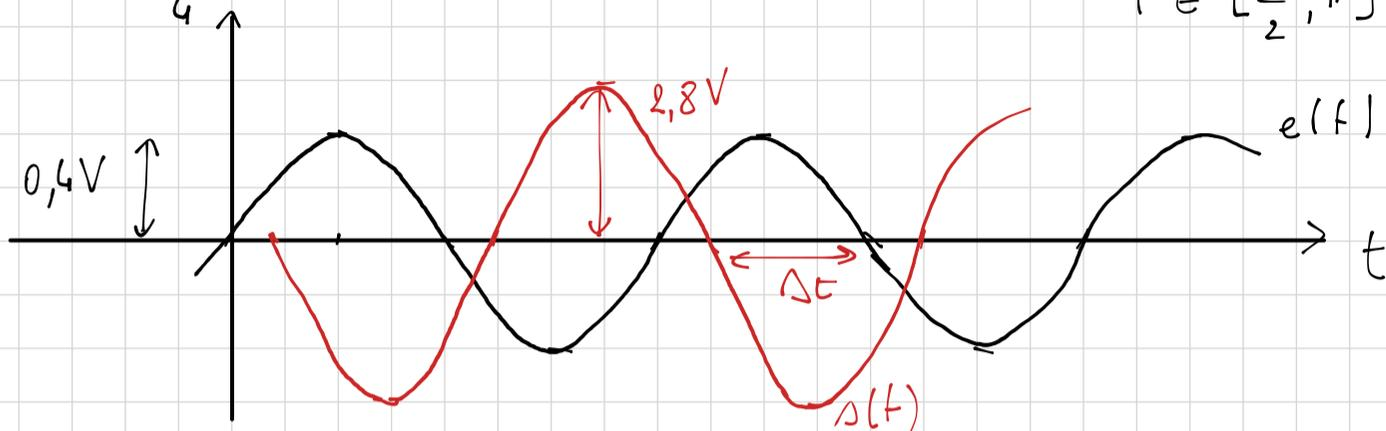
$$\varphi = 2\pi \frac{\Delta t}{T} \Rightarrow \Delta t = T \frac{\varphi}{2\pi} = T \times \frac{3\pi}{8\pi} = \frac{3}{8} T$$
