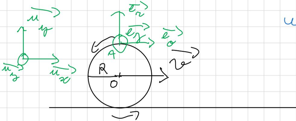
$$\omega = \frac{2\pi}{T}, \quad v = \frac{2\pi R}{T}, \quad R\omega = v$$
