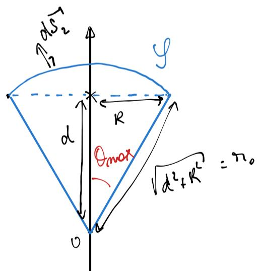
$$\begin{aligned} \vec{B}_1 \cdot d\vec{S}_2 &= \vec{B}_1 \cdot r_0^2 \sin\theta d\theta d\varphi \vec{\mu}_r \\ &= \frac{\mu_0 M}{4\pi r_0^3} r_0^2 \sin\theta \cdot 2\cos\theta d\theta d\varphi \end{aligned}$$
