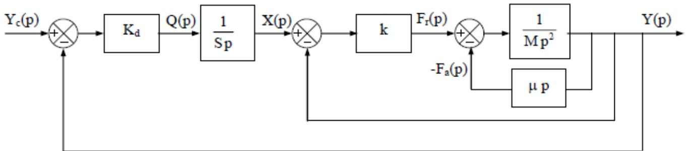
$$3 - \frac{Y(p)}{F_r(p)} = \frac{1}{Mp^2} \frac{1}{1 + \frac{\mu p}{Mp^2}} = \frac{1}{Mp^2 + \mu p} \quad \text{d'où} \quad H_1(p) = \frac{Y(p)}{X(p)} = \frac{k}{1 + \frac{k}{Mp^2 + \mu p}} = \frac{k}{Mp^2 + \mu p + k}$$
