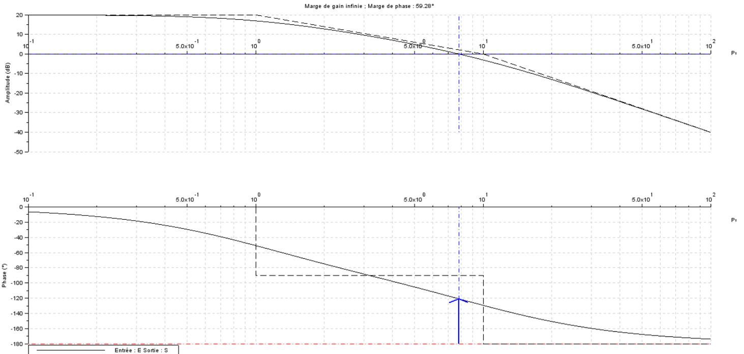
$$\mathbf{Q2} - \text{FTBF} = \frac{\frac{10}{11}}{1 + \frac{11}{110}p + \frac{1}{110}p^2} \quad \text{GS} = \frac{10}{11} \quad \omega_o = 10.5 \text{ rad/s } m = 0.52$$
