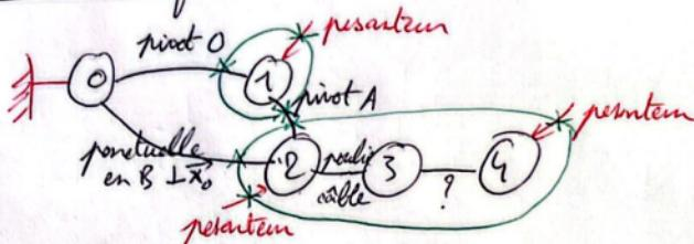
$$2. \quad \{T_{0 \rightarrow 1}\} = \begin{Bmatrix} X_{01} \\ Y_{01} \\ 0 \end{Bmatrix}; \quad \{T_{0 \rightarrow 2}\} = \begin{Bmatrix} X_{02} \\ Y_{02} \\ 0 \end{Bmatrix}_B \quad X_{02} < 0 \text{ car } 0 \rightarrow 2$$
