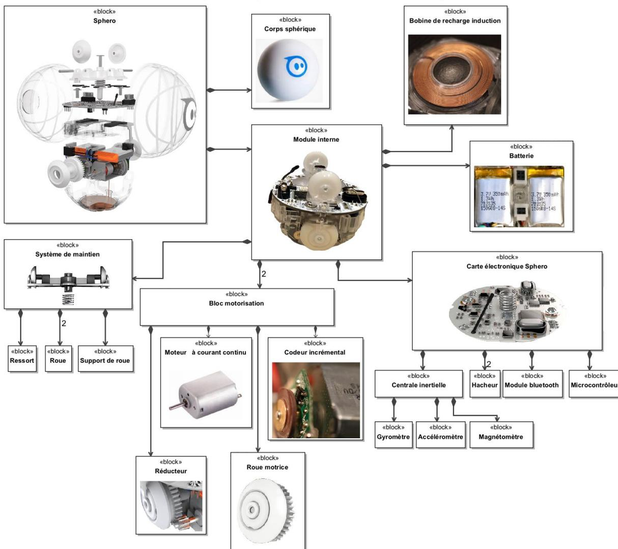
Figure 8 Diagram of block definition of the Sphero
