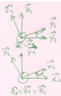
3.  $\vec{v}(P/O) = \dot{\lambda} \vec{y}_o - L \dot{\beta} \vec{y}_2 + L \sin \beta \dot{\alpha} \vec{x}_1$
