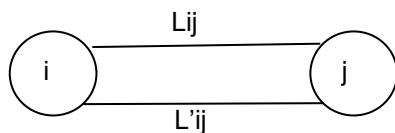
$$\{Vj/i\} = \begin{pmatrix} p_{ji} & 0 \\ q_{ji} & 0 \\ r_{ji} & 0 \end{pmatrix} \text{ et } \{V'j/i\} = \begin{pmatrix} p'_{ji} & 0 \\ q'_{ji} & 0 \\ r'_{ji} & w'_{ji} \end{pmatrix} A$$
