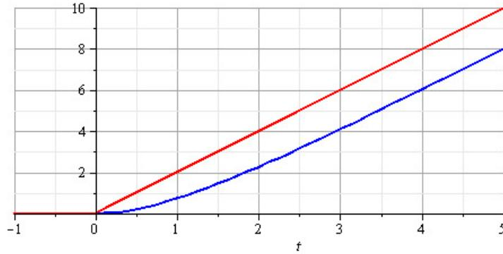
$$3. \quad s(t) + 2 \frac{ds(t)}{dt} + \frac{d^2s(t)}{dt^2} = e(t) \rightarrow S(p) + 2pS(p) + p^2S(p) = E(p) \rightarrow \boxed{\frac{S(p)}{E(p)} = \frac{1}{1+2p+p^2}},$$
