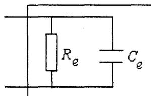
$$R_e = 1 \text{ M}\Omega ; C_e = 20 \text{ pF}$$
