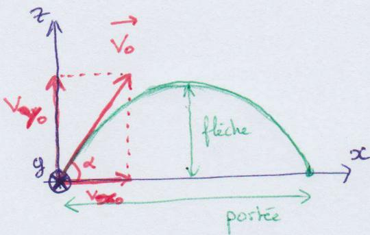
$$\vec{V}_0 = \begin{cases} V_{x0} = V_0 \cdot \cos(\alpha) \\ V_{y0} = 0 \\ V_{z0} = V_0 \cdot \sin(\alpha) \end{cases}$$
