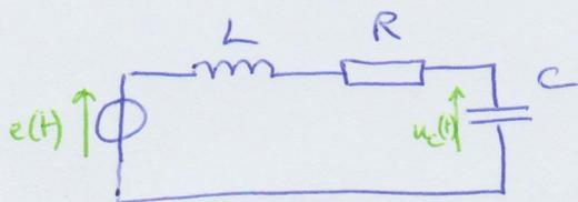
Q1 :  $\underline{u}_c(t) = \underbrace{U_c \cdot e^{j\varphi}}_{\underline{U}_c} e^{j\omega t}$  (on a  $e(t) = E_0 \cdot e^{j\omega t}$  donc  $E_0 = E_0$ )
