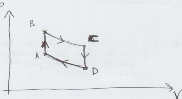
Q3 :  $A \rightarrow B : \left\{ \begin{array}{l} W_{A \rightarrow B} = 0 \\ \text{isochore} \end{array} \right.$
