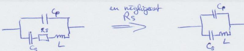
$$\underline{Z} = \frac{\frac{1}{jC_p\omega} \times \left(\frac{1}{jC_s\omega} + jL\omega\right)}{\frac{1}{jC_p\omega} + \frac{1}{jC_s\omega} + jL\omega} = \frac{\frac{1}{jC_p\omega} \times \frac{1}{jC_s\omega} (1 - LC_s\omega^2)}{\frac{C_s + C_p}{j(C_p \cdot C_s)\omega} (1 - L\left(\frac{C_s \cdot C_p}{C_s + C_p}\right)\omega^2)}$$
