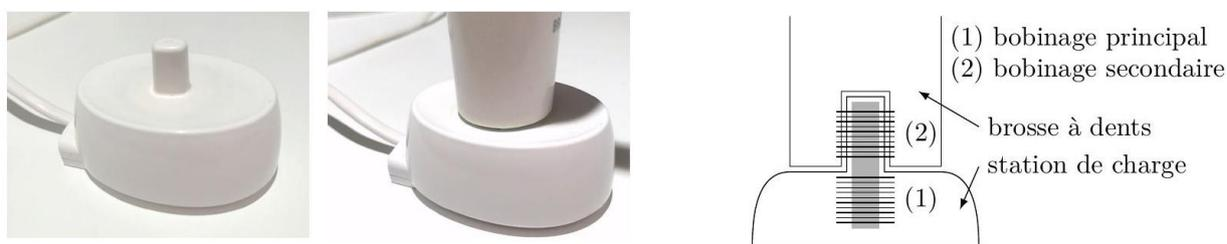
Figure 1: Station de charge
