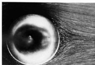
49. Sphere at  $R=25.5$ . Although it is not obvious, the flow is believed just to have separated at the rear at this Reynolds number, in contrast to the unseparated flow of figure 27. Aluminum dust is illuminated in water. Tanedá 1956b
