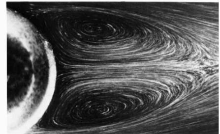
53. Sphere at  $R=118$ . The wake grows more slowly in asymmetric than plane flow. These photographs have shown that the length of the recirculating region is proportional to the logarithm of the Reynolds number, whereas it grows linearly with Reynolds number for a cylinder. Aluminum dust shows the flow of water. Tanedá 1956b
